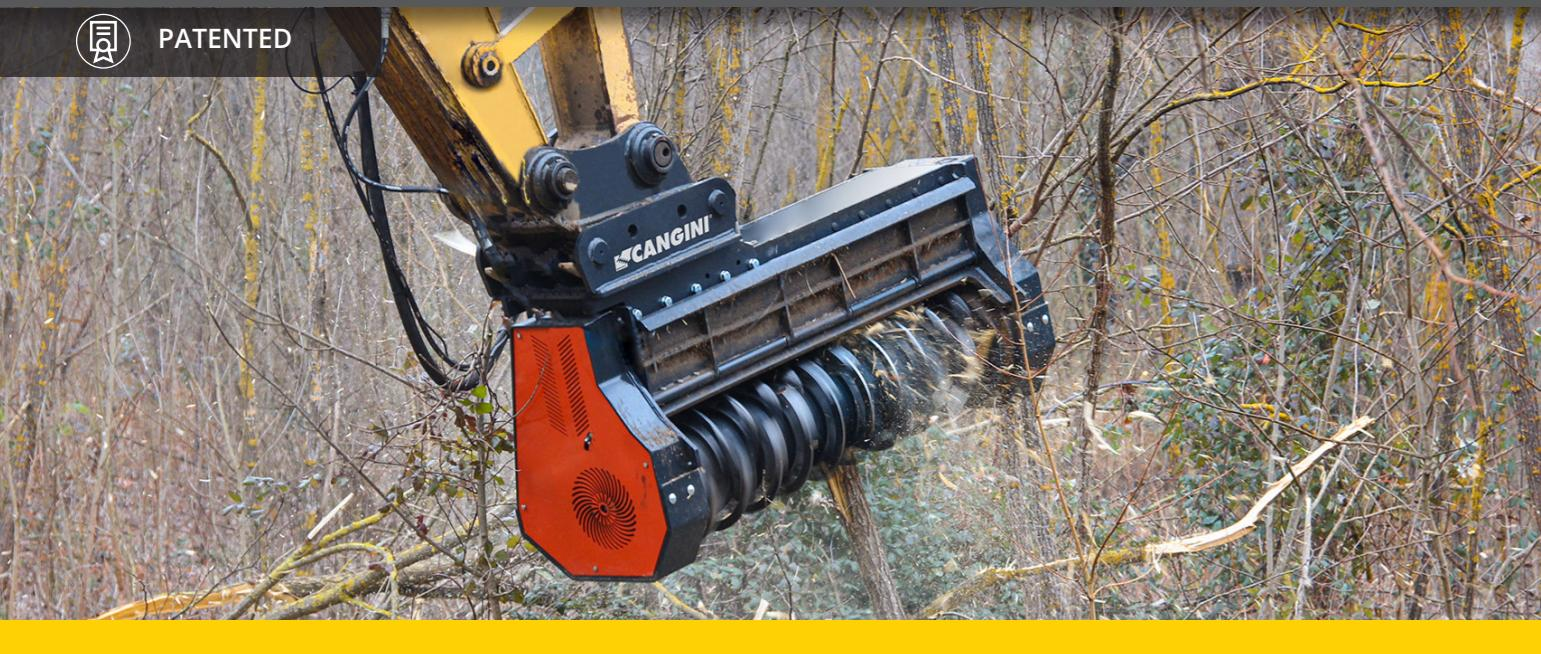
THE FORCE ONE FORESTRY FLAIL HEAD IS DESIGNED TO TACKLE THE HEAVIEST JOBS IN FORESTRY SUCH AS DEEP CLEARING OF WOODS AND FORESTS, MAINTENANCE OF WATERCOURSES AND RESTORATION OF AGRICULTURAL AREAS. IT IS EQUIPPED WITH A VARIABLE DISPLACEMENT PISTON ENGINE CAPABLE OF SUSTAINING VERY INTENSE WORK RHYTHMS. MAKING THE MOST OF THE HYDRAULIC PERFORMANCE OF THE OPERATING MACHINE AND TRANSFERRING THE MAXIMUM AVAILABLE POWER TO THE ROTOR.
