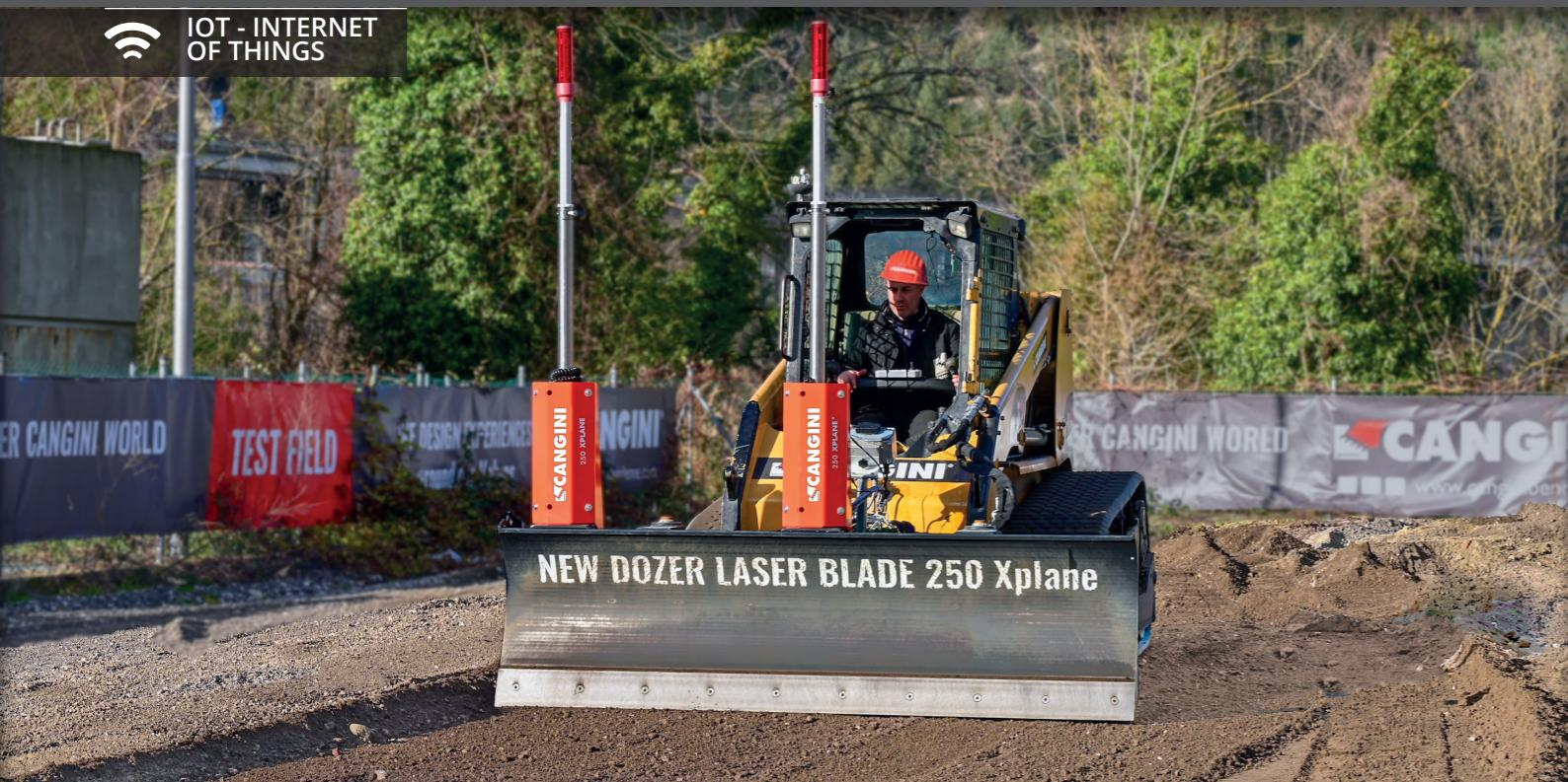
ALL MODELS OF THE XPLANE LASER DOZER BLADE ARE EQUIPPED WITH CANGINI'S IoT (INTERNET OF THINGS) TECHNOLOGY TO CONNECT TO THE CLOUD. THE CONTROL BOX, POSITIONED ON BOARD THE BLADE, AUTOMATICALLY COLLECTS ACTIVITY DATA TO PROVIDE A COMPLETE AND UP-TO-DATE VIEW OF THE EQUIPMENT'S ACTIVITY IN REAL TIME: WORKING HOURS, POSITION, MODE OF USE (AUTOMATIC OR MANUAL), DIAGNOSTICS.
