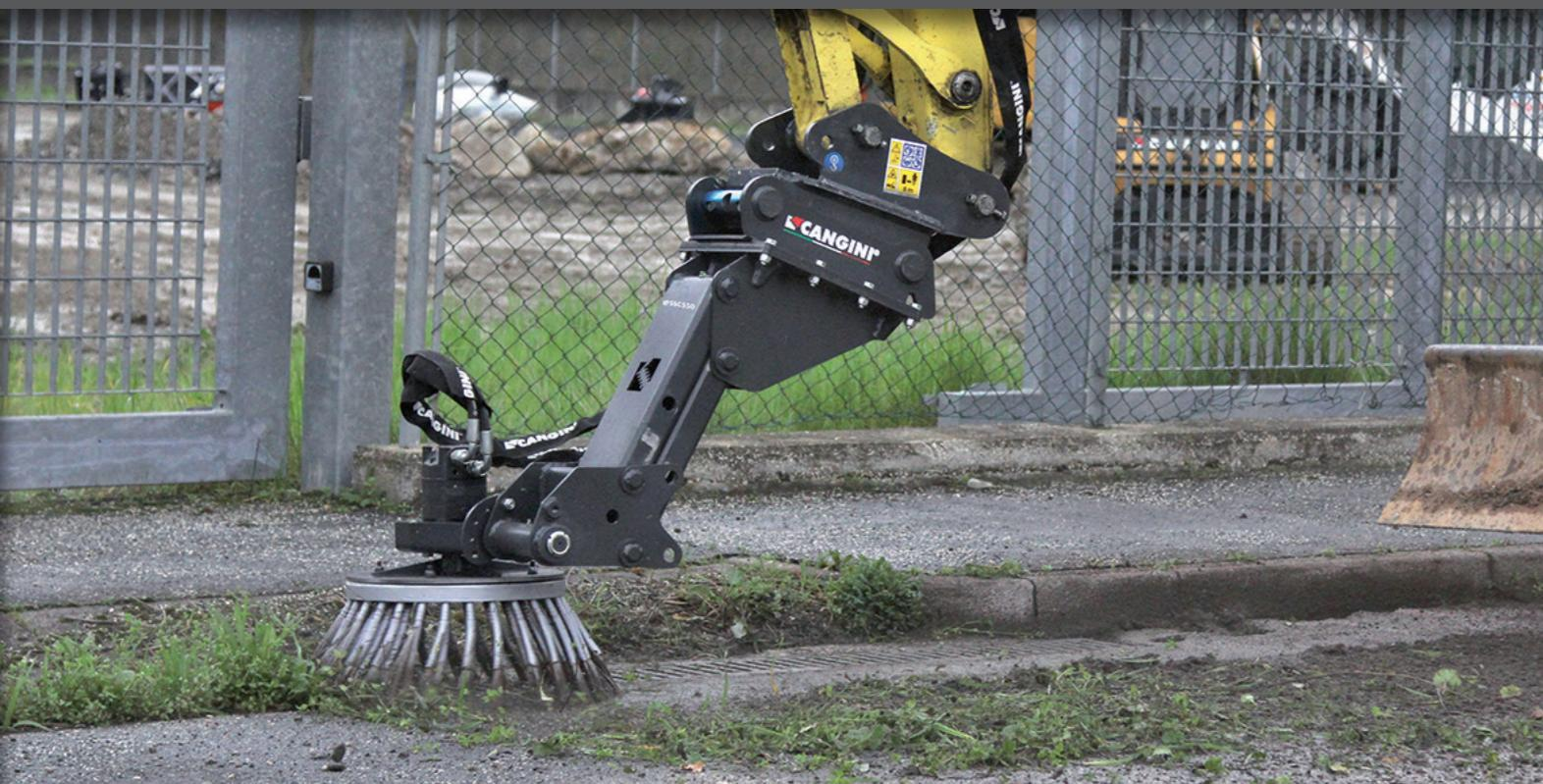
THIS BRUSH CAN BE APPLIED TO EXCAVATORS. IT IS MADE OF STEEL BRISTLES AND THEREFORE IDEAL FOR THE DEEP CLEANING AND WEED-REMOVAL OF CURBS, PLATFORMS AND BANKS, AND ASPHALTED AREAS. IT IS EQUIPPED WITH STANDARD FLOATING SYSTEM AND JOINT ON ITS HEAD THAT ENABLE THE BRUSH TO ADAPT TO ANY SURFACE. BOTH POSITIONING SYSTEMS CAN BE BLOCKED TO A FIX POSITION FOLLOWING THE UTILIZER'S NEEDS. IN ITS PPL BRISTLE VERSION THE BRUSH CAN CLEAN MORE DELICATE SURFACES WHERE THE WEED-REMOVAL IS NOT NECESSARY.
