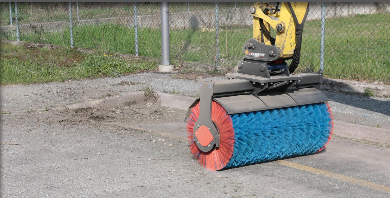
THE BROOM SWEEPER FOR EXCAVATORS IS SUITABLE FOR THE CLEANING OF HORIZONTAL AND VERTICAL SURFACES AND OF AREAS THAT MACHINES WITH FRONTAL ATTACHMENTS CANNOT REACH. IT IS EQUIPPED WITH STABILIZING SHOES TO SAFEGUARD BRUSHES WHEN THE BROOM IS SET TO THE GROUND. STANDARD THROTTLE VALVES AND PRESSURE RELIEF VALVES. THE DIRECT DRIVE ENGINE WITH DISK GEARBOX IS PLACED INSIDE THE BRUSH SHAFT TO REDUCE THE TOOL'S OPERATING OVERALL WIDTH.
