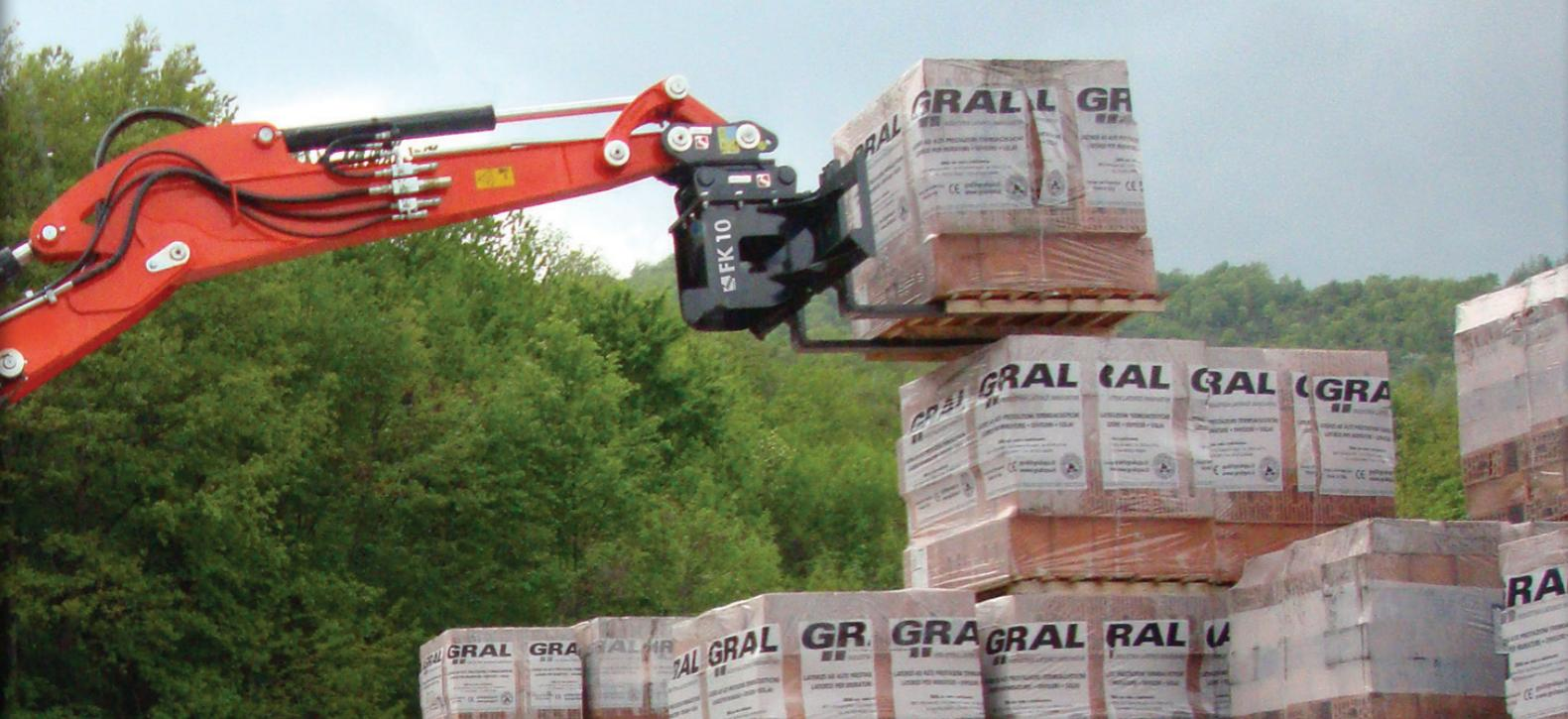
CETTE CONFIGURATION PERMET L'ACCROCHAGE AUX PELLES ET REND LE TABLIER APPROPRIÉ POUR LA MANUTENTION DES CHARGES DANS DE ZONES DURES D'ARRIVER AUTREMENT. CEPENDANT, IL FAUT VÉRIFIER QUE LA PELLE EST HOMOLOGUÉE POUR LE LEVAGE COMME L'EXIGE LA DIRECTIVE MACHINES.
