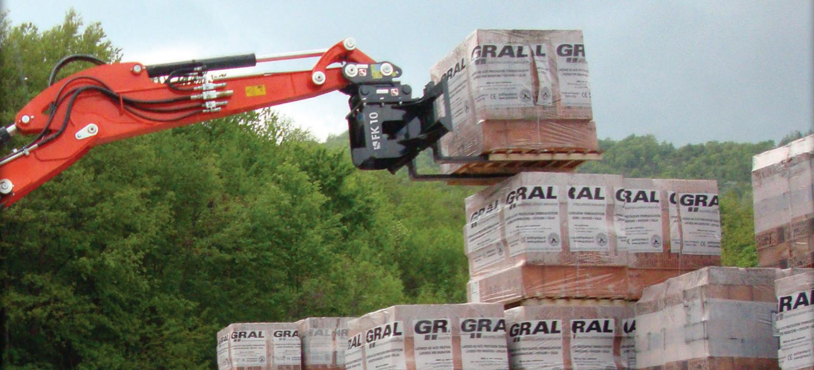
THIS CONFIGURATION ENABLES THE COUPLING TO EXCAVATORS MAKING IT SUITABLE FOR THE HANDLING OF LOADS IN HARD-TO-REACH AREAS. HOWEVER, IT IS IMPORTANT TO CHECK THAT THE EXCAVATOR IS COMPLIANT FOR LIFTING IN ACCORDANCE WITH THE MACHINERY DIRECTIVE.
