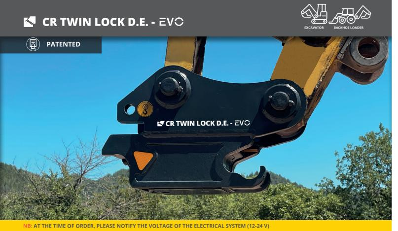
THE CR TWIN LOCK D.E. EVO REPRESENTS A TECHNOLOGICAL LEAP FORWARD IN EXCAVATOR QUICK COUPLER DESIGN, COMBINING SEVERAL INNOVATIVE TECHNOLOGIES IN A SINGLE PRODUCT, SUCH AS A HIGH-STRENGTH CAST BODY, DUCTED LUBRICATION, PATENTED "VISUAL CHECK" COUPLING DISPLAY AND UNI EN 474-1:2022 COMPLIANT FALL ARREST SYSTEMS.
