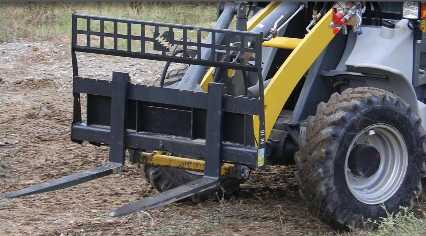
LE TABLIER FRONTAL PERMET L'ACCROCHAGE À CHARGEUSES COMPACTES, CHARGEUSES SUR PNEUS, TÉLESCOPIQUES ET TRACTOPELLES. EQUIPÉ D'UNE PROTECTION DE SÉCURITÉ CONTRE LE RENVERSEMENT DES CHARGES PENDANT L'UTILISATION, UNIQUEMENT DANS LES FOURCHES APPLIQUÉES AUX CHARGEUSES COMPACTES ET MINI-CHARGEUSES COMPACTES.
