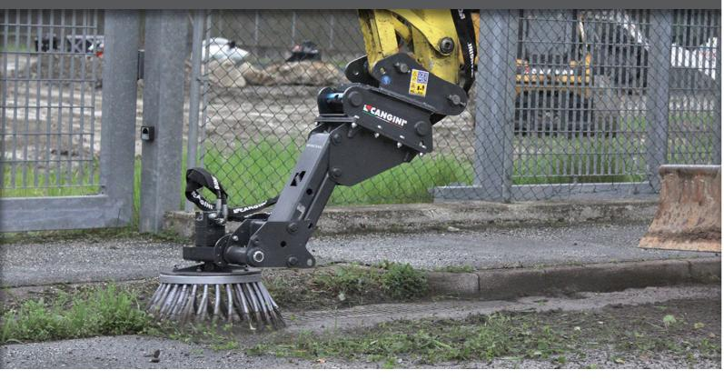
THIS BRUSH CAN BE APPLIED TO EXCAVATORS. IT IS MADE OF STEEL BRISTLES AND THEREFORE IDEAL FOR THE DEEP CLEANING AND WEED-REMOVAL OF CURBS, PLATFORMS AND BANKS, AND ASPHALTED AREAS. IT IS EQUIPPED WITH STANDARD FLOATING SYSTEM AND JOINT ON ITS HEAD THAT ENABLE THE BRUSH TO ADAPT TO ANY SURFACE. BOTH POSITIONING SYSTEMS CAN BE BLOCKED TO A FIX POSITION FOLLOWING THE UTILIZER'S NEEDS. IN ITS PPL BRISTLE VERSION THE BRUSH CAN CLEAN MORE DELICATE SURFACES WHERE THE WEED-REMOVAL IS NOT NECESSARY.
