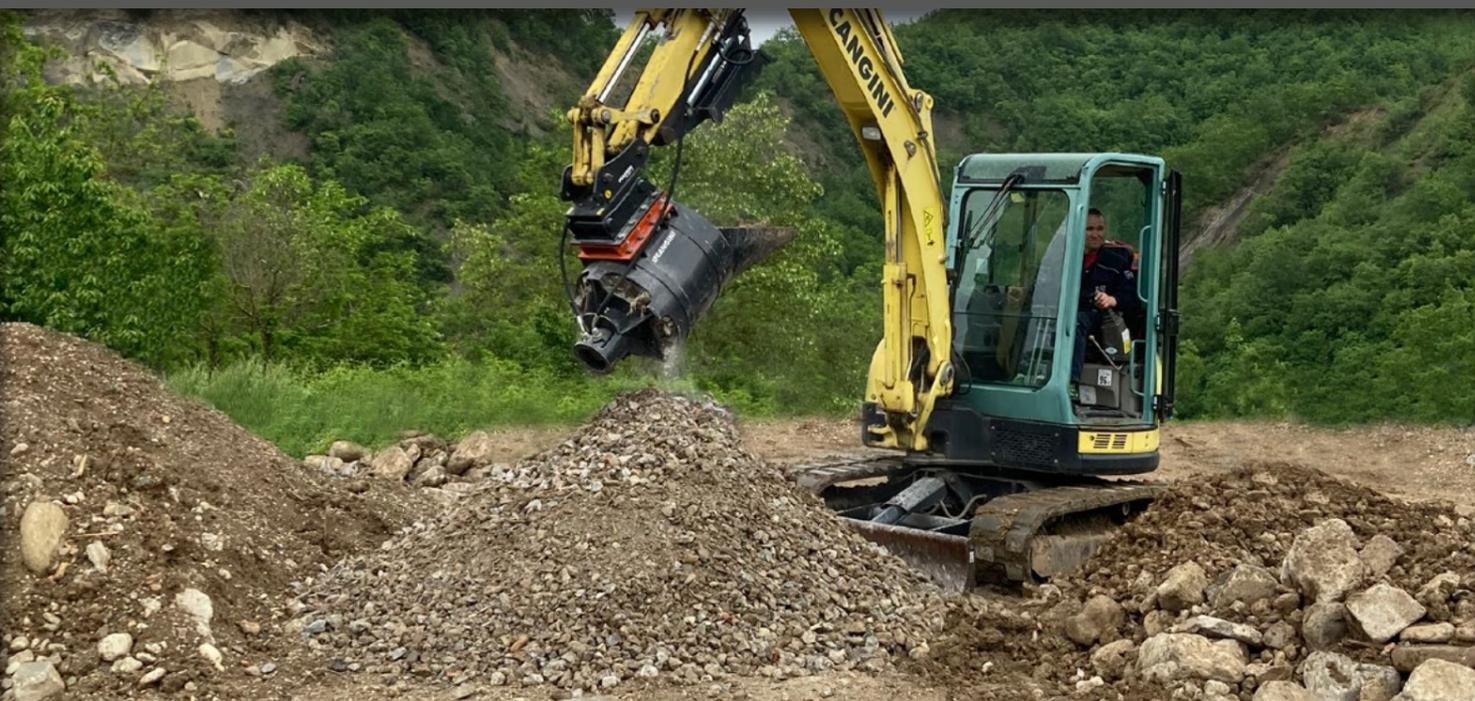
LE GODET CONCASSEUR DC FACILITE LE RETRAITEMENT ET LE RECYCLAGE DES GRAVATS ET DES DÉBRIS DE CONSTRUCTION DE PETIT VOLUME EN AGRÉGATS UTILISABLES. IL PERMET UN CONCASSEMENT JUSQU'À UNE TAILLE D'ENVIRON 40-70 MM. IL EST IDÉAL POUR DES APPLICATIONS TELLES QUE LA POSE DE FONDATIONS, LE PAVAGE DE TALUS ET DE COURS, L'AMÉNAGEMENT PAYSAGER, LES ROUTES OU COMME COUCHE DE BASE SOUS LE BÉTON COULÉ.
