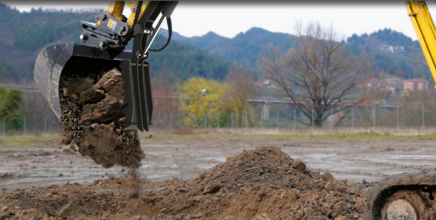
SOUDE SUR LE BRAS, LE POUCE GRT CANGINI FACILITE LA PRISE DE MATÉRIAUX ROCHEUX, TRONCS ET AUTRES, FAISANT OFFICE DE PINCE. UNE FOIS COMPLÈTEMENT RÉTRACTÉ, IL PERMET LE FONCTIONNEMENT NORMAL DU GODET, FACILITANT AINSI LE TRAVAIL DE L'OPÉRATEUR.
