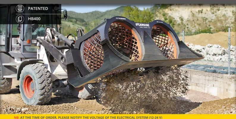
THE NEW MULTISCREENING BUCKET FOR FRONTAL COUPLING, WITH TWO ROTARY DOUBLE DRUMS COUPLED IN A SINGLE FRAME, IS SUITABLE FOR SELECTION DUTIES ON TURNED SOILS AND RESULTING MATERIALS. THE MATERIAL SIZE CHANGE, FROM A MINIMUM OF 25 MM TO A MAXIMUM OF 65 MM (1 - 2,4 IN), IS HYDRAULICALLY CONTROLLED FROM THE CAB WITHOUT REPLACING ANY MECHANICAL PART AND CONSIDERABLY REDUCING THE WORKING TIMES.
