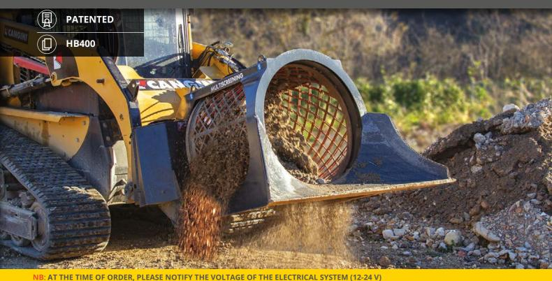
THE MULTISCREENING BUCKET WITH THE NEW ROTARY DOUBLE DRUM CONCEPT FOR FRONTAL COUPLING AND MACHINES UP TO 14 TONS (30865 LB) IS SUITABLE FOR SELECTION DUTIES ON TURNED SOILS AND RESULTING MATERIALS. THE MATERIAL SIZE CHANGE - FROM 25 TO 60 MM (1 - 2,4 IN). - IS CONTROLLED DIRECTLY AND HYDRAULICALLY FROM THE CAB WITHOUT REPLACING ANY MECHANICAL PART THUS REDUCING THE WORK TIMES CONSIDERABLY.
