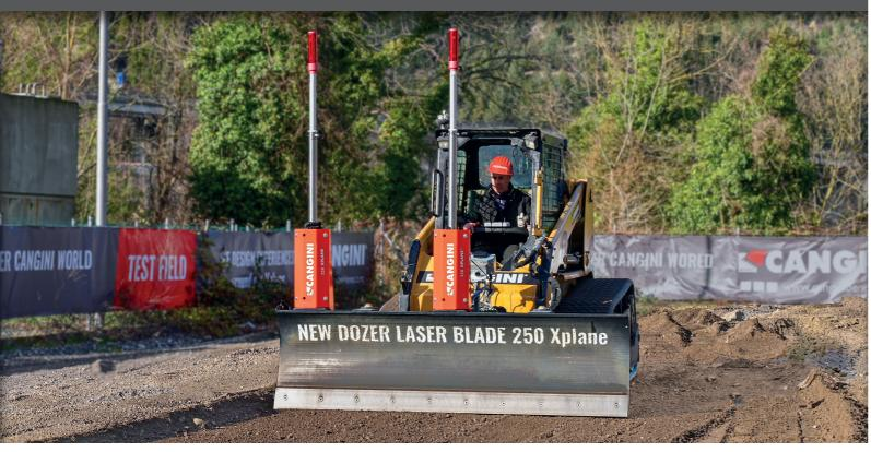
THE DOZER LASER SYSTEM HAS THE SAME STRENGTH AND VERSATILITY AS THE STANDARD DOZER. IT ALSO ENABLES CREATION OF A CONTROLLED PLANE THANKS TO A DUAL-SLOPE LASER TRANSMITTER. THE SIGNAL IS RECEIVED AND PROCESSED BY THE ELECTRONICS ON BOARD THE BLADE, WHICH ACTS DIRECTLY ON THE PROPORTIONAL ELECTRIC CONTROL VALVE TO PILOT THE BLADE. THE OPERATOR TERMINAL IN THE CAB COMMUNICATES WITH THE CONTROL BOX VIA WIRELESS NETWORK. THIS MEANS NO WIRES TO INTERFERE WHEN THE CAB DOORS ARE SHUT.
