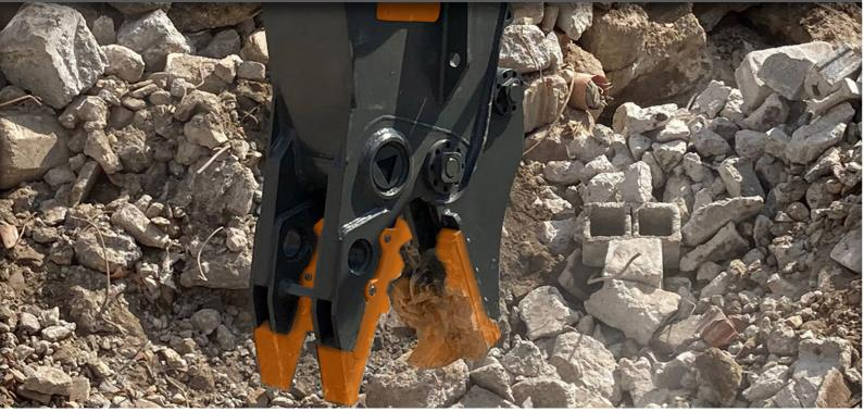
THE DEMOLITION ROTATING PULVERISERS GATOR HAS BEEN DESIGNED FOR PRIMARY AND SECONDARY DEMOLITION INCLUDING THE CRUSHING OF PREVIOUSLY DEMOLISHED MATERIAL ON THE GROUND IN ORDER TO REDUCE IT FOR THE DISPOSAL PROCESS AND RECYCLING. SUITABLE FOR CUTTING AND CRUSHING HEAVY MATERIAL SUCH AS CONCRETE WITH METAL REINFORCEMENT AND STEEL STRUCTURES. IT IS HIGHLY RESISTANT THANKS TO ITS STRUCTURE DESIGNED TO INCREASE ITS CRUSHING FORCE.
