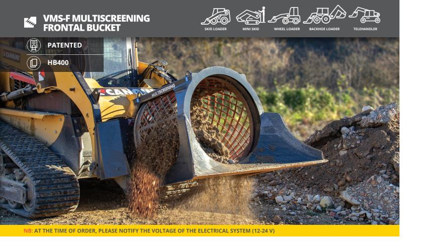
THE MULTISCREENING BUCKET WITH THE NEW ROTARY DOUBLE DRUM CONCEPT FOR FRONTAL COUPLING AND MACHINES UP TO 14 TONS (30865 LB) IS SUITABLE FOR SELECTION DUTIES ON TURNED SOILS AND RESULTING MATERIALS. THE MATERIAL SIZE CHANGE - FROM 25 TO 60 MM (1 - 2,4 IN). - IS CONTROLLED DIRECTLY AND HYDRAULICALLY FROM THE CAB WITHOUT REPLACING ANY MECHANICAL PART THUS REDUCING THE WORK TIMES CONSIDERABLY.
