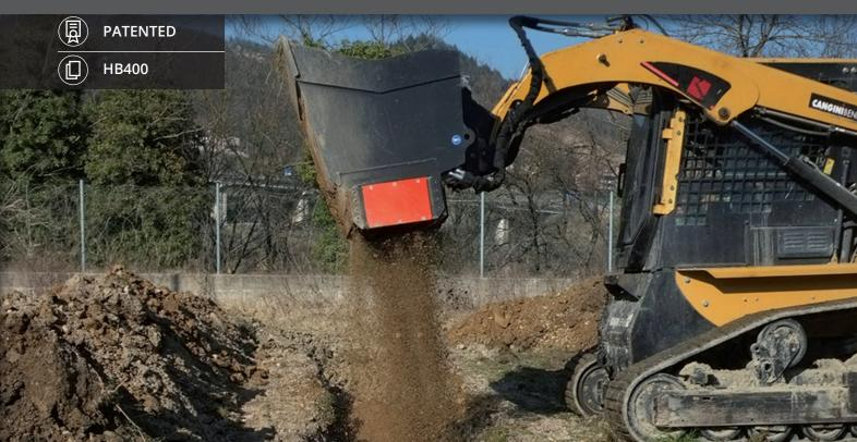
IT GRADES MATERIALS FROM DEMOLITION, DIGGING AND EARTH-MOVING WORKS. IT IS IDEAL ALSO FOR THE MIXING OF TERRAIN AND PEAT. THE CORE-ELEMENT IS AN HYDRAULIC SIEVE WITH ROTATING HB400 KNIVES. THE MATERIAL THICKNESS CAN VARY FROM 0 TO 20 (0 - 0,8 IN) AND FROM 0 TO 35 (0 - 1,4 IN) WITH A STANDARD EQUIPMENT.
