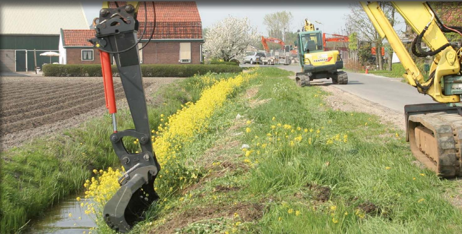
PARTICULIÈREMENT INDIQUÉ POUR DE TRAVAUX DE CURAGE OÙ LE RAYON D'ACTION DE LA MACHINE, EN CONFIGURATION STANDARD, N'EST PAS SUFFISANT. EST FOURNI COMME "QUASI MACHINE" SELON L'ANNEXE II-B DE LA DIRECTIVE 2006/42/CE. IL DEVRA ÊTRE DECLARÉ CONFORME CE APRÈS SON COUPLMENT À LA MACHINE ET AVANT SA MISE EN SERVICE.
