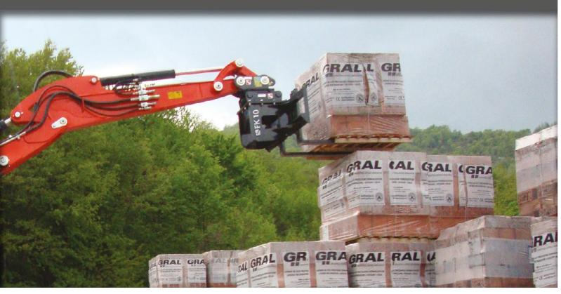
THIS CONFIGURATION ENABLES THE COUPLING TO EXCAVATORS MAKING IT SUITABLE FOR THE HANDLING OF LOADS IN HARD-TO-REACH AREAS. HOWEVER, IT IS IMPORTANT TO CHECK THAT THE EXCAVATOR IS COMPLIANT FOR LIFTING IN ACCORDANCE WITH THE MACHINERY DIRECTIVE.
