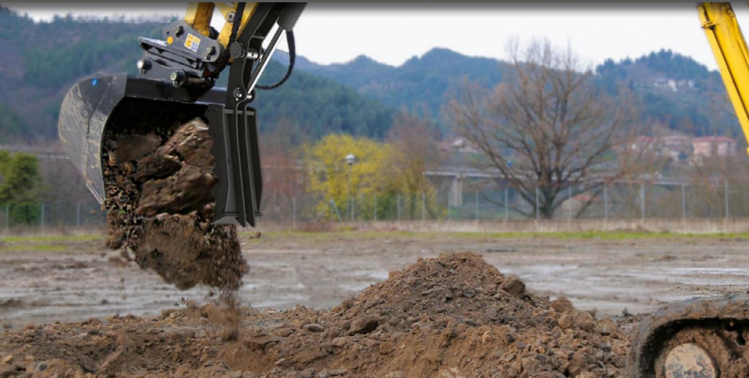
SOUDE SUR LE BRAS, LE POUCE GRT CANGINI FACILITE LA PRISE DE MATERIAUX ROCHEUX, TRONCS ET AUTRES, FAISANT OFFICE DE PINCE. UNE FOIS COMPLETEMENT RETRACTE, IL PERMET LE FONCTIONNEMENT NORMAL DU GODET, FACILITANT AINSI LE TRAVAIL DE L'OPERATEUR. LORS DE LA COMMANDE, LA FAISABILITE DE L'APPLICATION DOIT ETRE VERIFIEE AFIN D'EVITER TOUT DYSFONCTIONNEMENT DE L'OUTIL.
