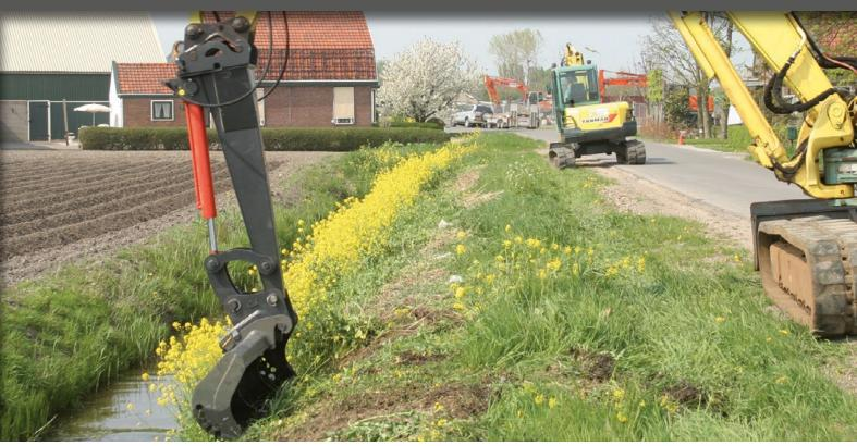
PARTICULARLY SUITED TO OPERATIONS IN AREAS WHERE THE MACHINE'S STANDARD RANGE OF ACTION IS NOT SUFFICIENT. THE EXTENSION ARM IS SUPPLIED AS A "PARTLY COMPLETED MACHINERY" CERTIFICATION IN ACCORDANCE WITH THE ANNEX II-B OF THE 2006/42/EC MACHINERY DIRECTIVES. ITS EC COMPLIANCE WILL BE DECLARED AFTER IT HAS BEEN ATTACHED TO THE MACHINE AND BEFORE ITS REGULAR USE.
