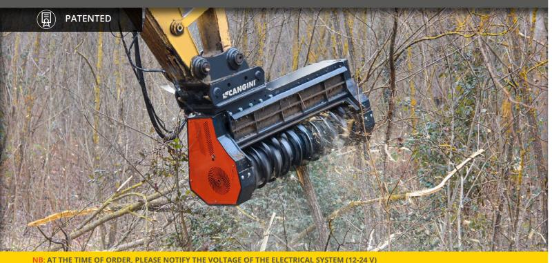
THE FORESTRY MULCHER HAS BEEN DESIGNED TO MANAGE THE HEAVIEST WORKLOADS: THE DEEP CLEARING OF WOODS AND FORESTS. IT IS EQUIPPED WITH A PISTON ENGINE TO RUN AT THE MOST INTENSE WORK PACE. THE EXCAVATOR-TYPE MULCHER CAN REACH THE NARROWEST AREAS.
