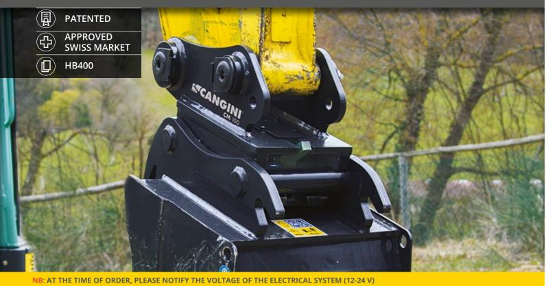
THE **REVERSIBLE** CM SICURMATIC QUICK COUPLER IS EQUIPPED WITH THE MOST ADVANCED SAFETY SYSTEMS: THE FRONT SAFETY SYSTEM THAT IS ACTIVATED WHEN THE PINS COME OUT; THE FORK WITH ITS NEW DOUBLE-NOTCH PROFILE; THE VISUAL INDICATOR THAT SHOWS THE OPERATOR THE LOCKING STATUS FROM THE CAB. SIDES ARE MADE IN HB400.
