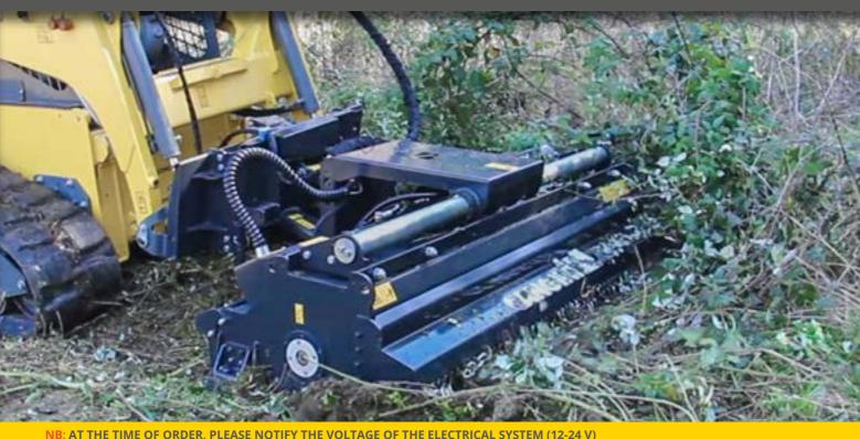
THE FRONT TC MULCHER IS MADE OF A DOUBLE BODY IN ORDER TO INCREASE THE TOOL'S RESISTANCE TO SHOCKS. IT'S EQUIPPED WITH MECHANICAL (HYDRAULIC UPON REQUEST) SIDE-SHIFTING AND VERTICAL FLOATING SYSTEMS, ADJUSTMENT TO THE HORIZONTAL PLANE OF ± 10°, ALSO EQUIPPED WITH BYPASS, PRESSURE RELIEF AND FLOW-DIVIDER VALVES, STANDARD Y BLADES WITH INTERMEDIATE KNIFE OR HAMMERS.
