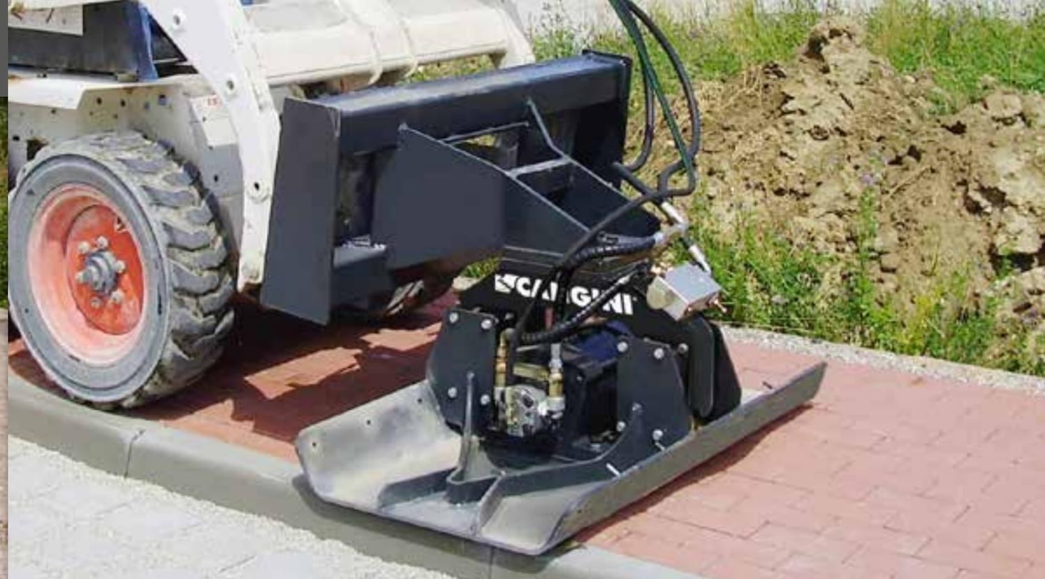
CONÇUE POUR COMPACTER TOUTES LES SURFACES, LA PLAQUE VIBRANTE EST PARTICULIÈREMENT UTILE POUR LE COMPACTAGE DE MATÉRIAUX DESTINÉS AU PAVAGE, AU REVÊTEMENT DES ROUTES ET À LA CRÉATION DE PISTES CYCLABLES ET DE TROTTOIRS. EN ASSURANT UNE BASE SOLIDE, HOMOGENÈME ET DURABLE.
