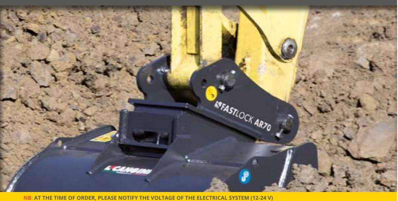
THE AR FAST LOCK PATENTED QUICK COUPLER ENABLES THE FAST LOCKING AND UNLOCKING OF THE ATTACHMENT TOOLS, CONSIDERABLY REDUCING THE TIME FOR THEIR REPLACEMENT. THE MECHANICAL VERSION IS PROVIDED WITH A SEMI-AUTOMATIC SYSTEM THAT REQUIRES THE MANUAL INTERVENTION WHEN THE TOOL HAS TO BE RELEASED. BOTH THE LOCKING AND THE SAFE BLOCKING OF THE NEW TOOL ARE AUTOMATIC OPERATIONS. IN THE HYDRAULIC VERSION THESE FUNCTIONS ARE MANAGED DIRECTLY FROM THE CAB.
